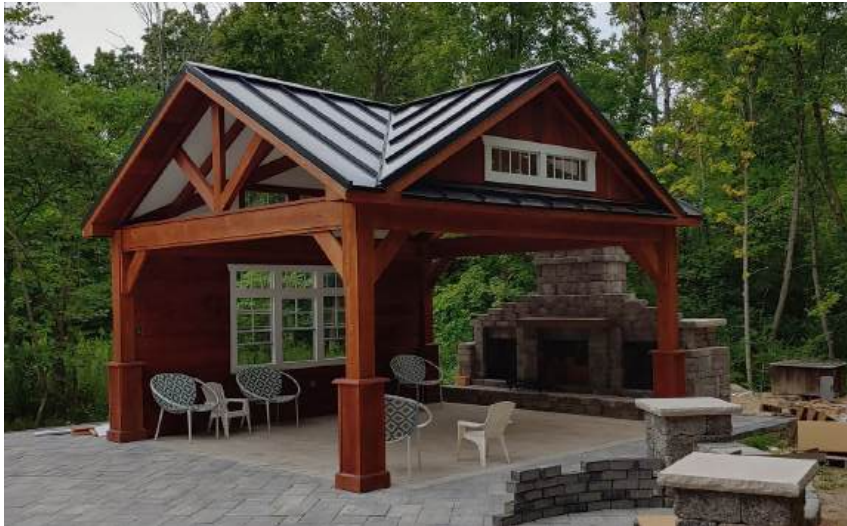
14x16 wood A-frame with open gables with braces, functional A-frame dormer with transom windows, standing seam metal roof, privacy wall with windows, traditional deluxe post trim & rustic cedar stain
